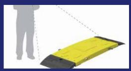
1. Check top surface of Road Plate for signs of damage.
